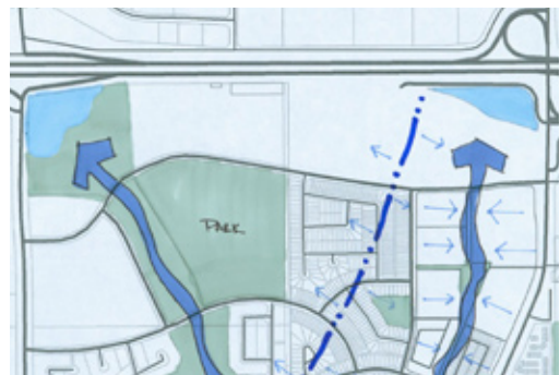
Additional runoff is conveyed to natural stormwater facilities off-site
